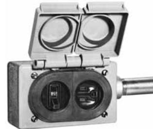
Spring doors open wide for easy plug insertion and cover assembly (covers shown in open position for illustration only). This view shows gaskets that protect plugs. Gasket on bottom of cover prevents entry of moisture into device box (see gasket description).
