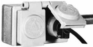
Typical application with NEMA configuration receptacle and plug, mounted on an FS box. Gasket seals around plug, keeping out moisture and dirt. Spring door closes automatically when plug is withdrawn to protect receptacle.
