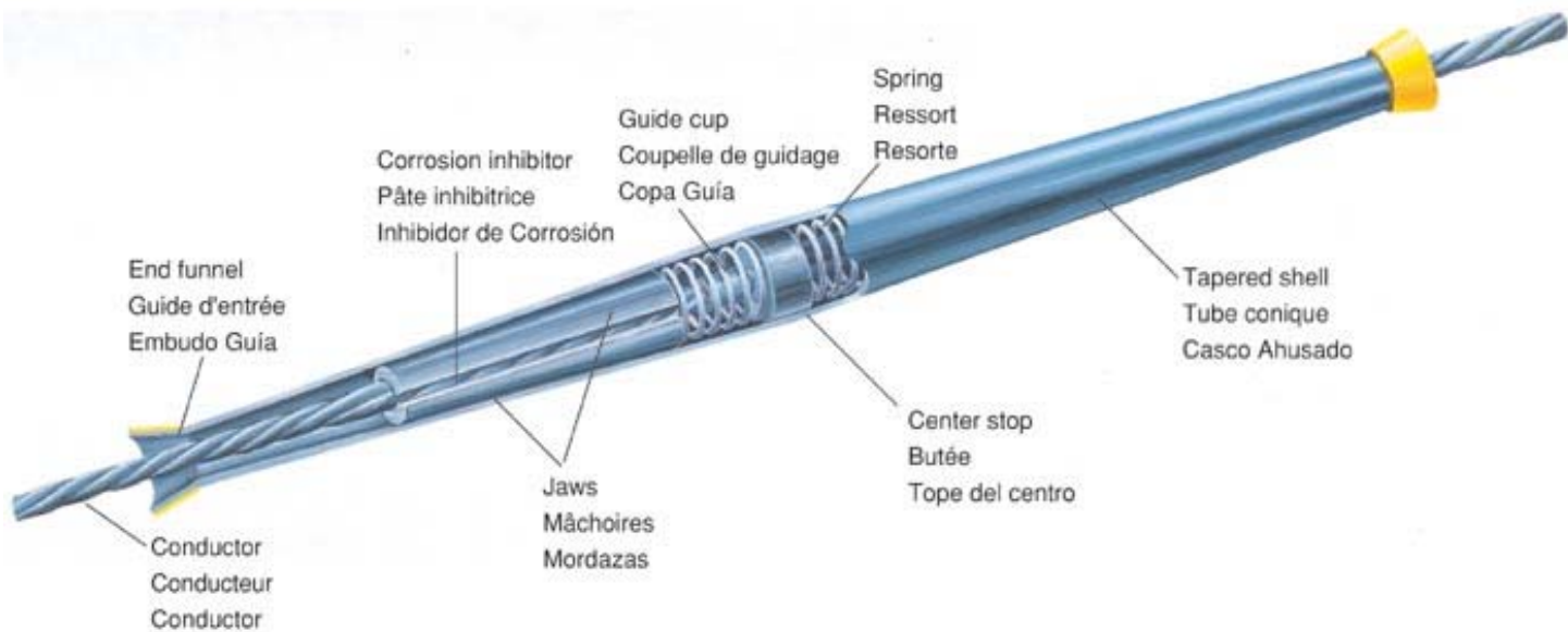
Inside an Automatic Splice.
