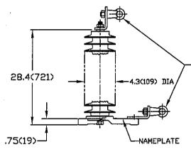
CLAMP TYPE LINE & GROUND TERMINALS SUITABLE FOR USE WITH CU DR AL CONDUCTOR (25(6) TO (81(21) DIA
