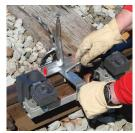
• Used to remove the slag from the crucible area of the mold after making a ERICO CADWELD connection
