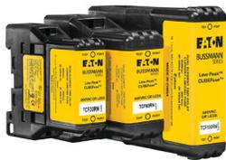
All 30, 60 and 100 A CUBEFuse holders dovetail together to create the desired number of poles. Each holder accepts CUBEFuse amp ratings up to its rating. E.g., the 60 amp holder will accept a CUBEFuse from 1 to 60 A.
