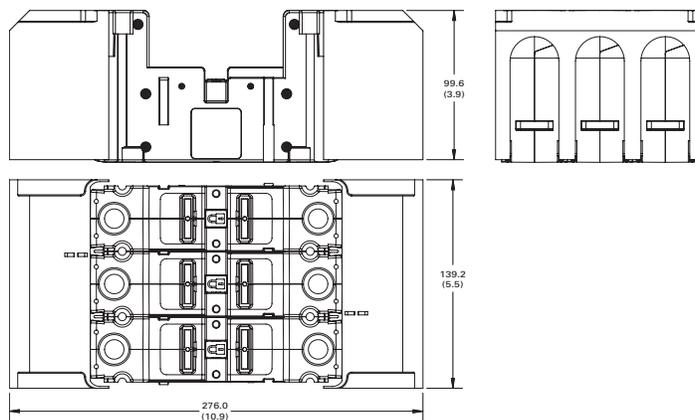
3-pole ganged 400 A holder with installed shroud
