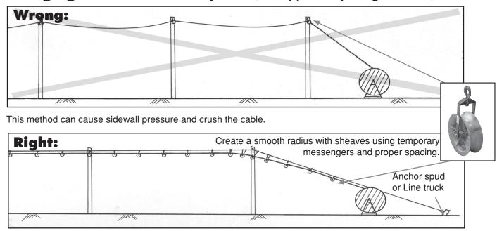
This method will support and distribute all bearing loads for successful cable installation.
