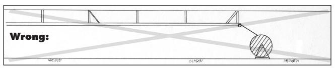
This method can cause sidewall pressure and crush the cable at the leading point. Lack of rollers will increase drag creating more tension.
