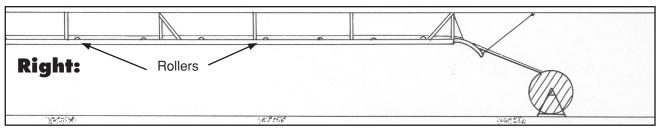
Use a large multi-wheel conveyor to distribute sidewall pressure. Lead and exit wheels must meet minimum cable bend. Use tray rollers to eliminate cable drag.
