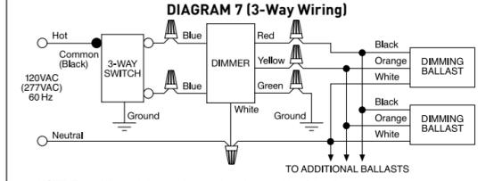
NOTE: The 3-Way switch must be wired on the line side of the dimmer.
