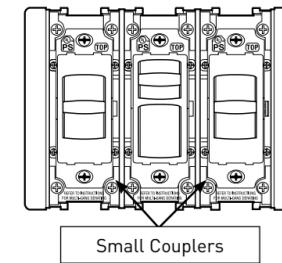
6. Tighten the mounting screws, insert the label, attach the wall plate, and restore power to the circuit.
