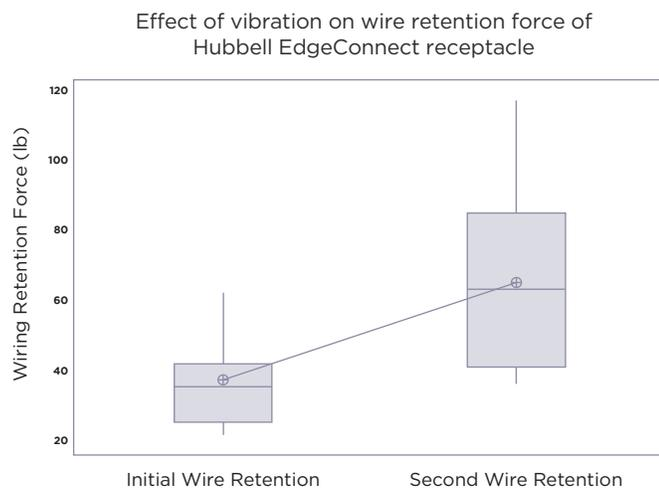
Upon installation, a 10 AWG THHN stranded wire required 40 lb of force to disengage. After exposure to vibration per the UL standard, 65 lb of force was required to disengage.
