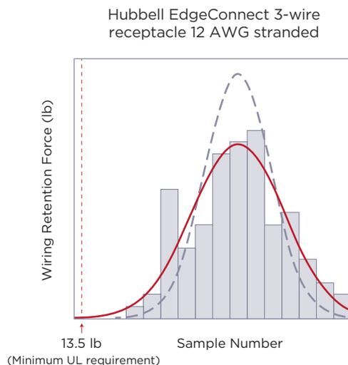
Compared to the UL minimum requirement for wire retention, EdgeConnect screwless termination offers superior strength.
