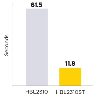
Seconds saved with screwless termination: **49.7** per piece
