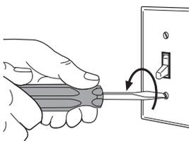
Turn screws counterclockwise to loosen.
