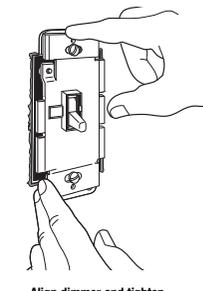
Align dimmer and tighten screws clockwise.
