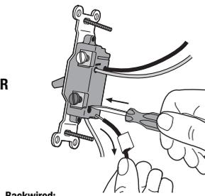
**Screw Terminals:** Turn screws counterclockwise to loosen.
