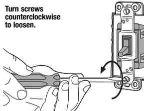
**Step 3** **Disconnect switch wires.**
