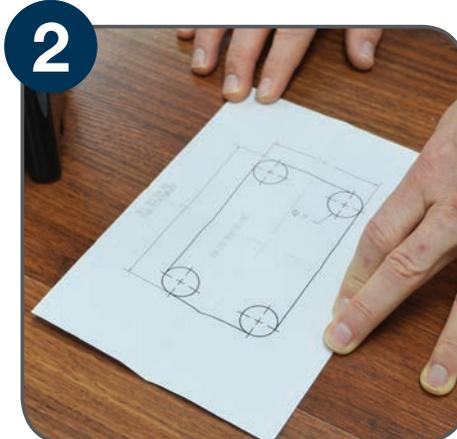
2 Once measured, place the installation template on the floor and cut a hole accordingly. A small drill, jigsaw, or hole saw can be used to precisely cut the hole required.
